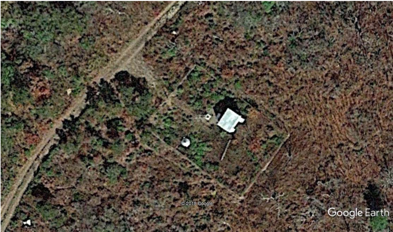
The Bald Knob site is an approximately 85' x 55' fenced compound with a guyed tower, equipment building, and an underground propane tank.
